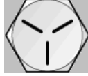
Figure 7 – Head View of Standard SAE Grade 5 Bolt, where the grade of ‘5’ is indicated by 3 radial lines
