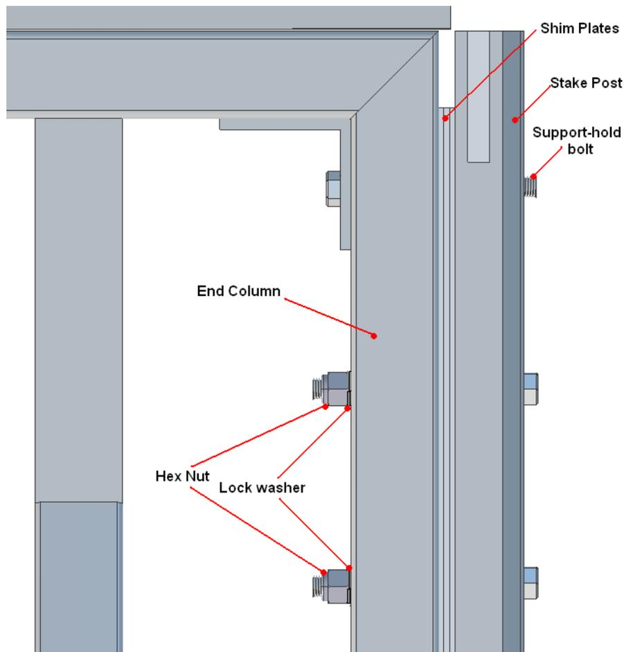
**Figure 6: Illustrated view of aligned and installed hex bolt/nut/lock washer components in lower two holes in Load Leveler's curb-side Stake Post-shim plating-end column series**
