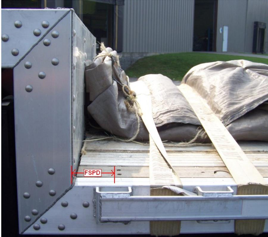
Figure 3: Measuring the distance from the drop deck wall to the center-line of the foremost lower deck side rail pocket
