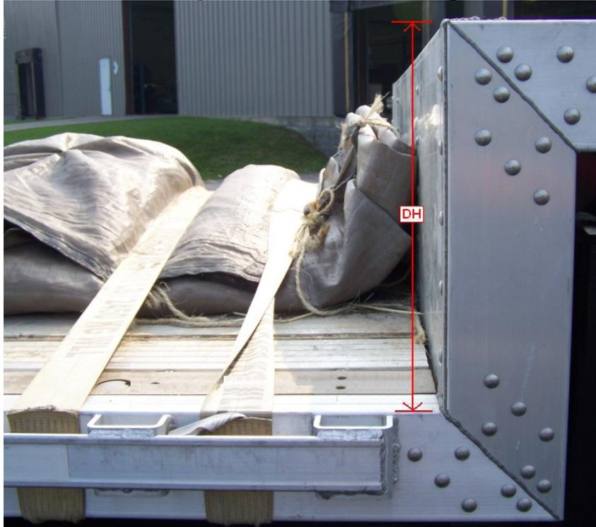
Figure 1: Measuring the overall height differential ("DH") between the upper and lower decks of your Trailer
