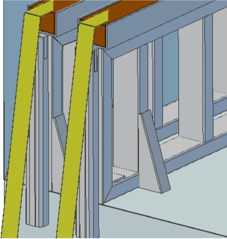
**Figure 10: Illustrated view of two Load Leveler units with a Ratchet Strap resting within each unit's top channel, and extending down along the ends**
