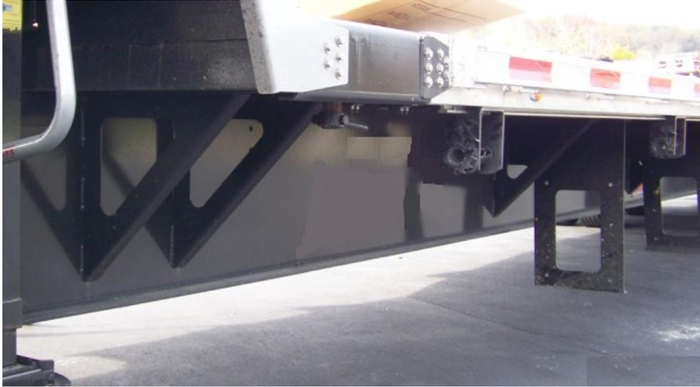
**Figure 6 – Perspective View of trailer frame Outriggers**
