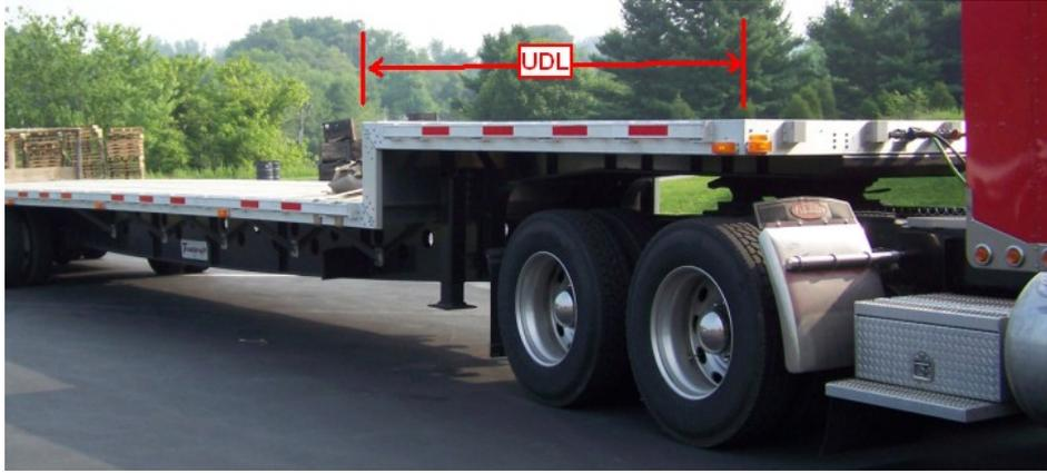
**Figure 2: Measuring the Trailer's upper deck length available for use (entire deck shown available in this view)**
